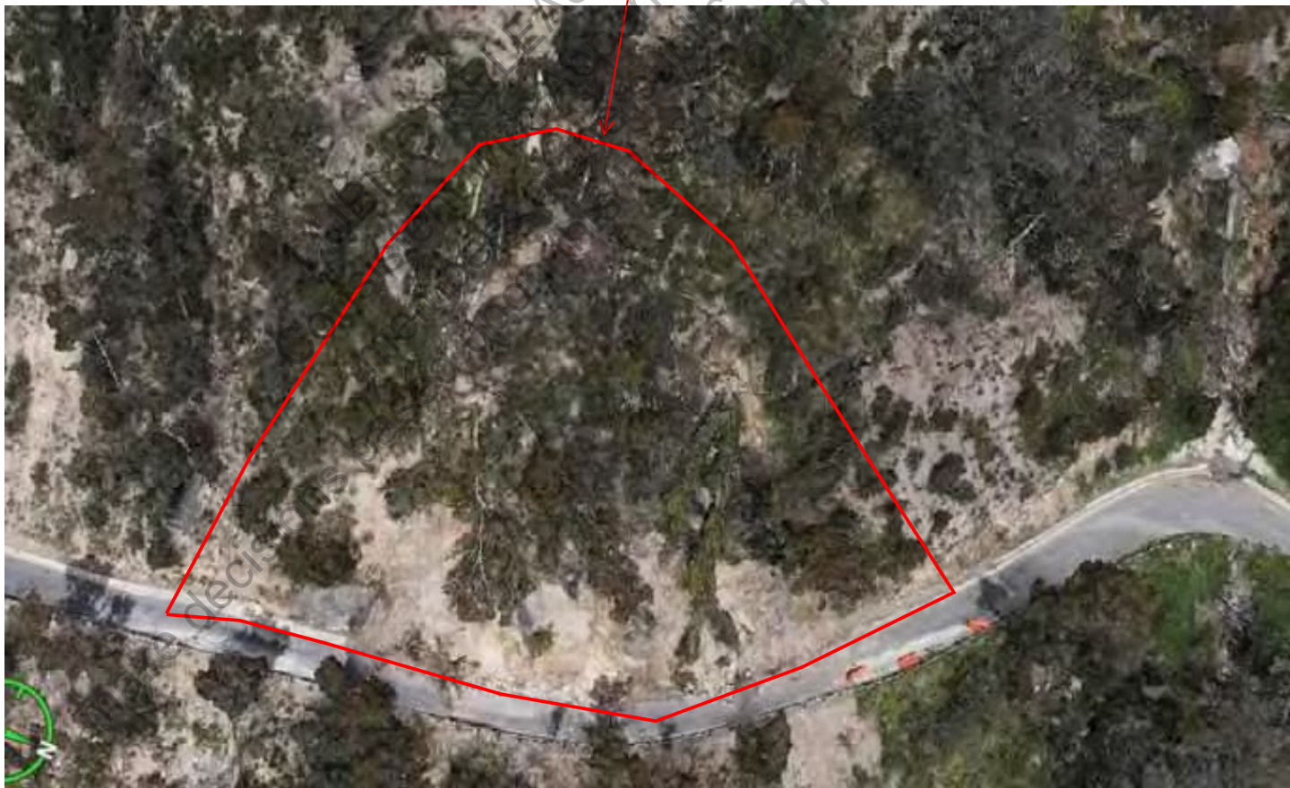
Example H2.1 Upslope Debris Slide Hazard, enlarging (Approx. 60 m wide, 60 m long)
