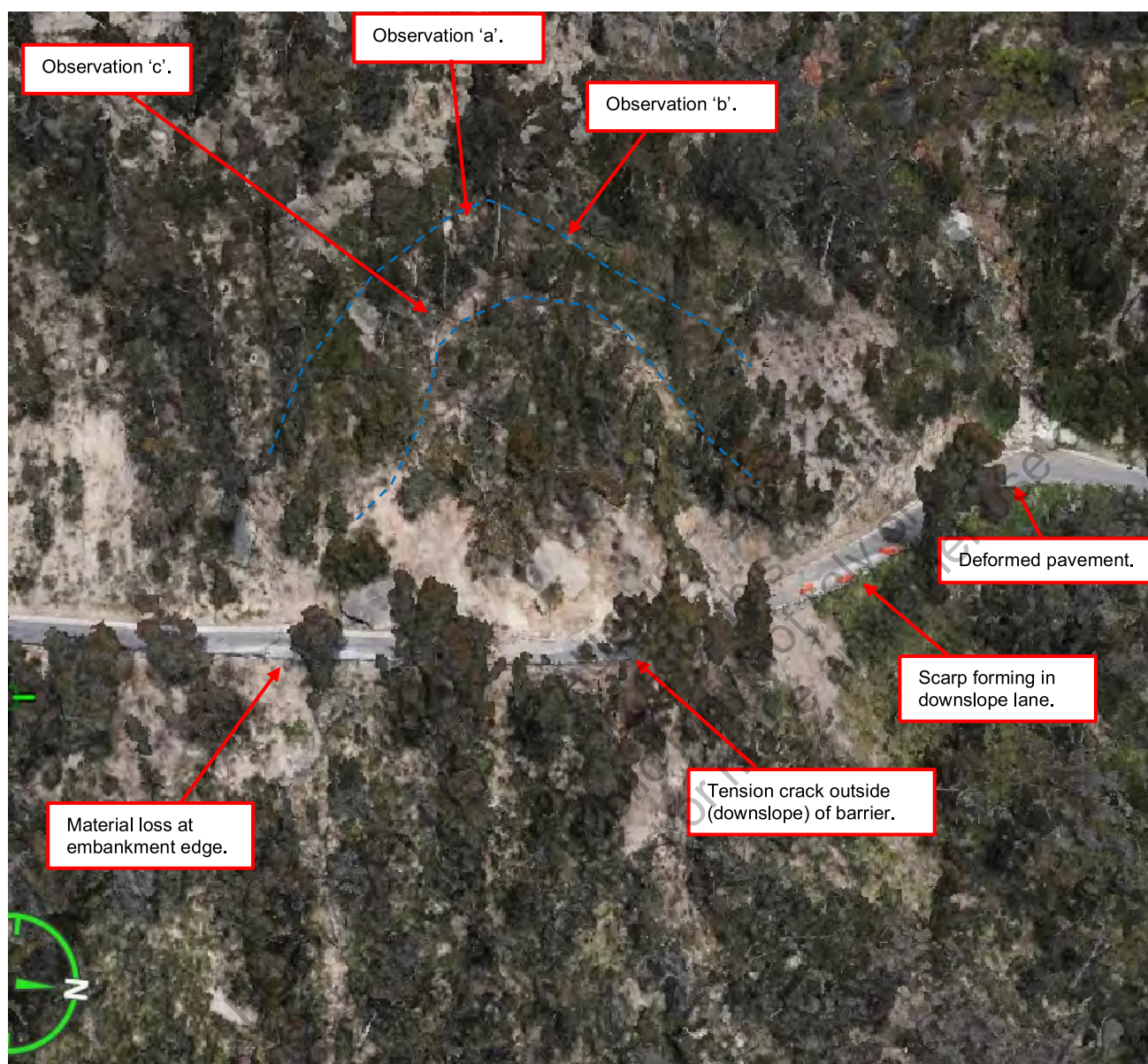
Figure 5 : Surface features corresponding with slope instability observed at Site 11, November 2022, annotated on 15.11.22 aerial photogrammetric survey.
