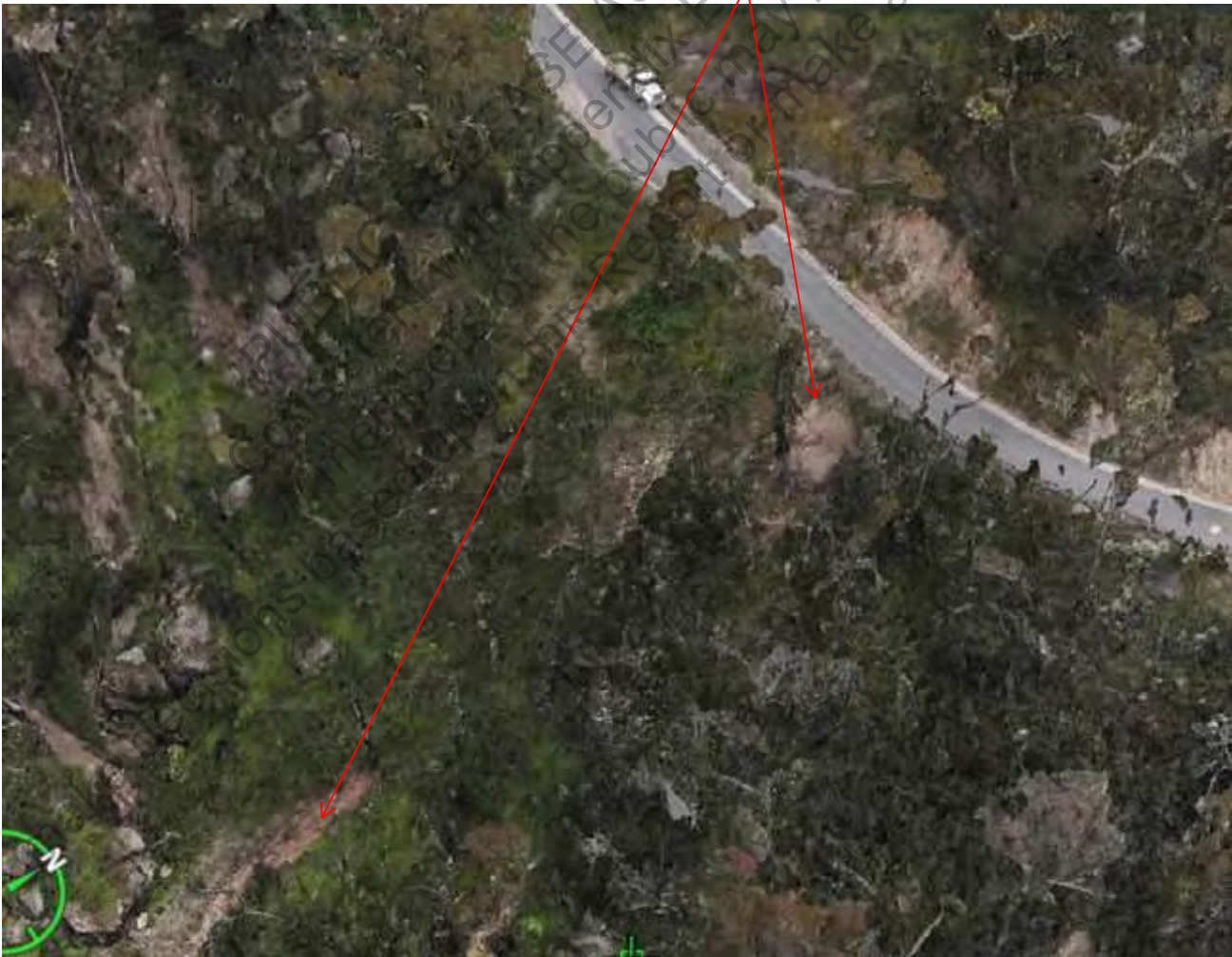
Example H3.1 Downslope Debris Flow Hazard, right flank (Approx. 5 m wide, 10-20 m long, 2 m deep)
