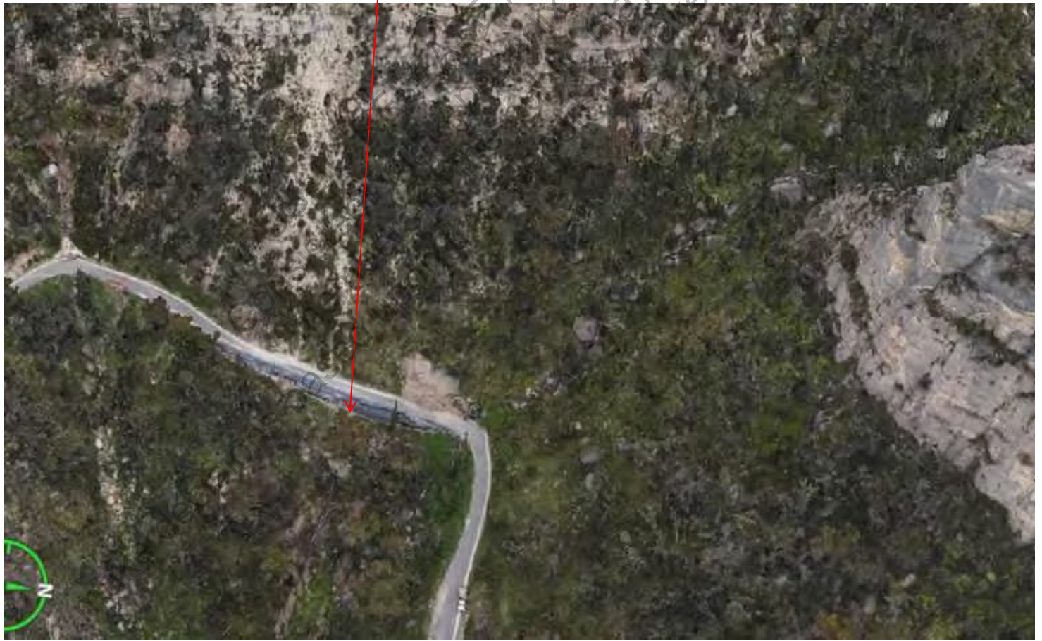
Example H3.2 Downslope Debris Slide Hazard, (Approx. 100 m wide)
