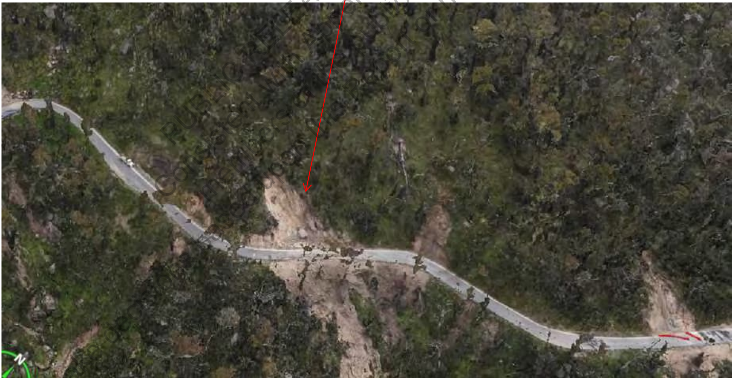
Example H2.1 Upslope Debris Flow Hazard, left flank (Approx. 40 m wide, 40 m long, 2 m deep)
